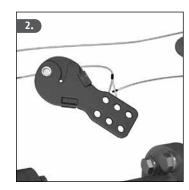
2. Thread the cable through the looped end of the lockout assembly. Tension the cable as tight as possible.
