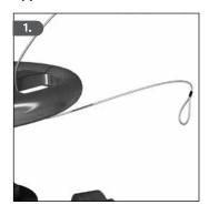
Pass the non-looped portion of the cable through or around all the components intended to be locked out.
