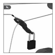
4. Squeeze the device closed and insert up to six padlocks.
